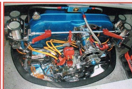
ABOVE, Miguel Girasol is mighty proud of his '78 Puma ... the Cat! RIGHT, Miguel, his brother Milton and friend Rodrigo, built this well-detailed 1914cc engine fitted with dual Weber 44 IDF carbs. Puma "flat-top" fan housing was powder-coated candy blue. LEFT, Puma factory alloy wheels measure 14x6 and 14x7, with front 185/65/14 and rear 205/70/14 tires.
